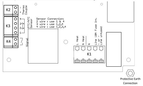
**K4:** Potential-free signal for external monitoring or control systems. The signal output should be connected as follows. The connection (NO contact potential-free) may be max. be connected with 45VDC and 50mA. The tap is to be inserted into the housing via the M12 cable gland and connected to the two signal terminals as per the picture. The connection (NO contact) is only activated when the setpoint and actual temperatures are the same or within the tolerances.
